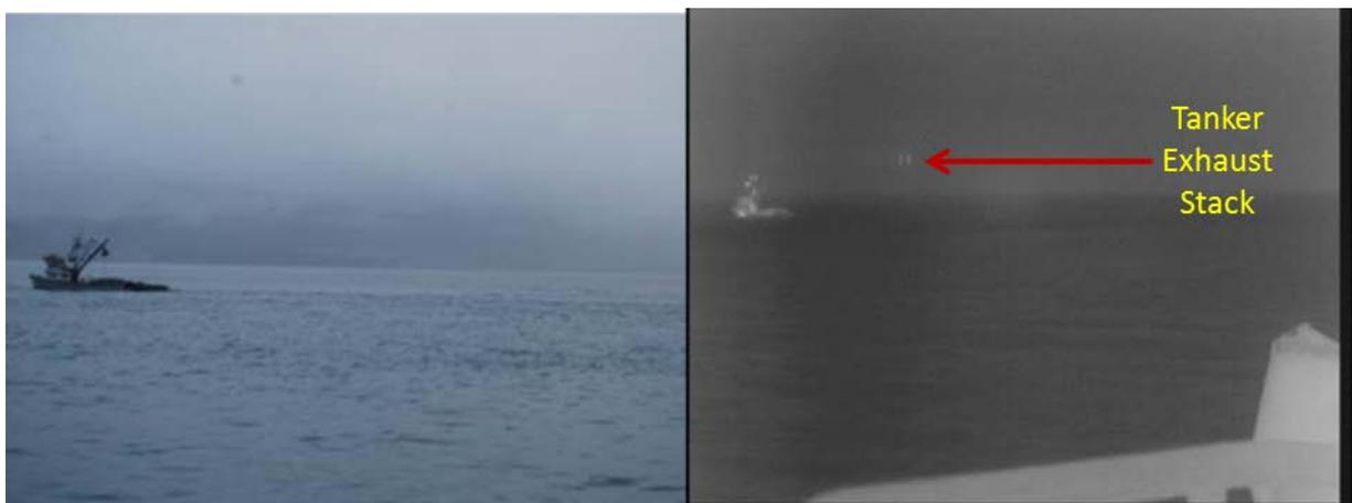
Note in Figure 2, we see not only the obvious fishing vessel in 10-14 micron LWIR (Long Wave Infrared), but also the engines and exhaust system of the Supertanker at the TAP (Trans Alaska Pipeline), which is more evident with a narrower field of view as shown in Figure 3, but still obscured by fog. With image fusion, the thermally hot pixels in the LWIR image can be overlaid on the visible image in a single image with proper image registration and resolution matching.
