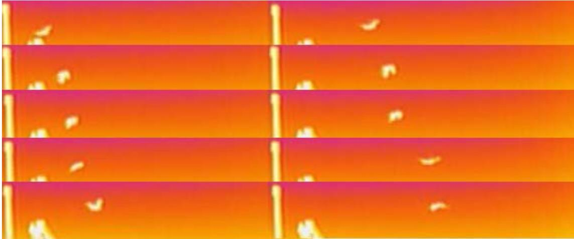
At this stage of SDMSI development, visible images were tested along with 10-14 micron LWIR, but not yet fused. Rather both were tested with the same object detection algorithms. For example, drone detection was evaluated using both LWIR and visible images in one combined test as shown in Figure 13.
