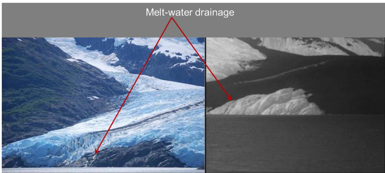
The use of LWIR and visible extends the spectral resolution at a common spatial and pixel resolution with much better temporal resolution than occasionally over flights by satellite remote sensing for field monitoring of geological locations of interest.
