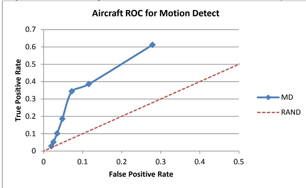
Figure 9 shows that simple motion triggered detection of aircraft results in detection better than random (the dashed diagonal shown on the ROC), but to detect more than 60% of all passing aircraft, the false positive rate with a sensitive threshold configuration is almost 30%. This same simple motion detector was also tested with flights of a DJI Inspire drone to determine detectability compared to aircraft. Figure 10 shows and ROC for this drone test.
